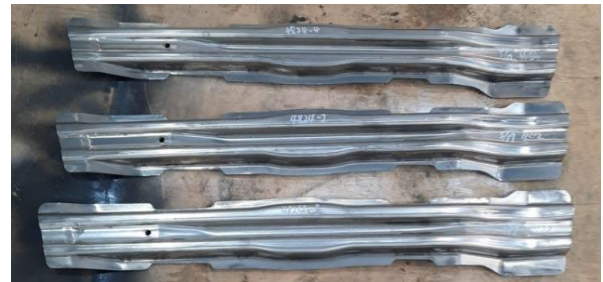
Fig.6. Hot forming 7075 door impact beams.
