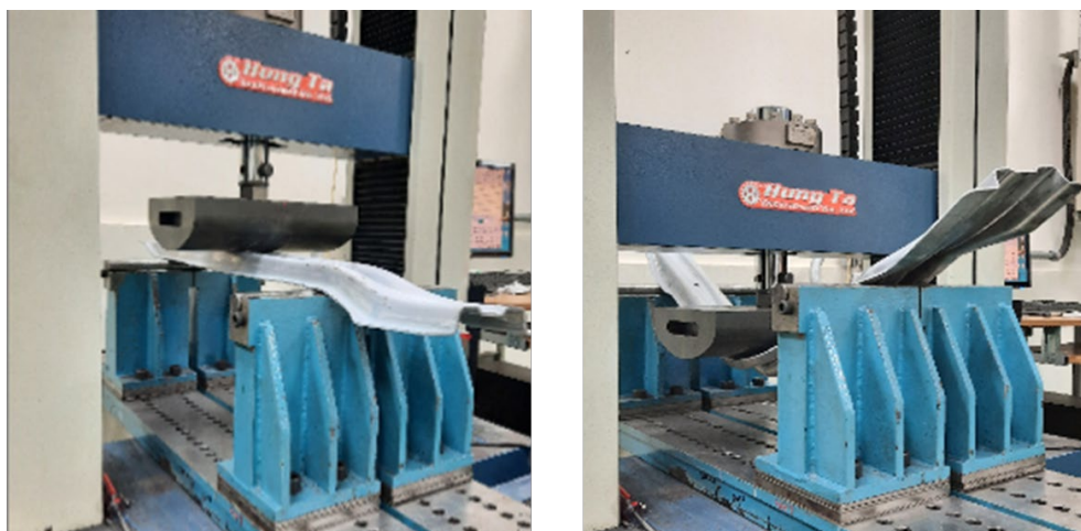
Fig.4. Schematic of three-point bending test.
